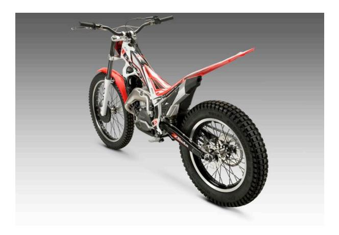
There are other new features for the EVO 250 2T and 300 2T in terms of the exhaust, which has a new and longer steel manifold and a new silencer, also longer at the end. This new configuration guarantees greater torque at low speeds, without sacrificing performance at high speeds, and noise reduction with a "fuller timbre".
