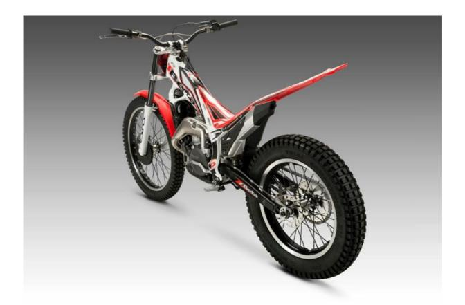
There are other new features for the EVO 250 2T and 300 2T in terms of the exhaust, which has a new and longer steel manifold and a new silencer, also longer at the end. This new configuration guarantees greater torque at low speeds, without sacrificing performance at high speeds, and noise reduction with a "fuller timbre".
